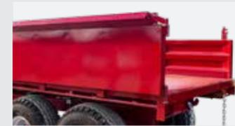
3mm two piece drop-in sides, with solid reinforcing posts for extra strength.
