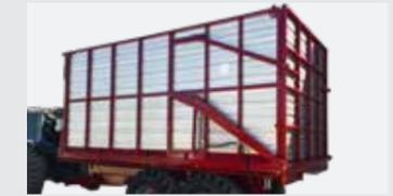
Optional silage cage with hydraulically opening rear door and drop-down front can be custom built to suit your requirements.
