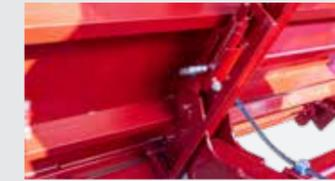
A clever rear pivot design gives high ground clearance and keeps the load centre well forward when the deck is raised, leaving weight on the drawbar. Tipping angles are up to 57° for a clean dump.
