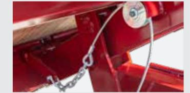
The adjustable automatic tailgate release is standard, tripping the tailgate at the desired deck height. It can be upgraded to a hydraulic trip mechanism.
