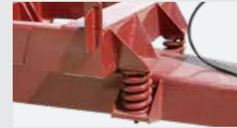
Heavy duty 10mm pressed steel drawbar provides strength in critical load areas and a tight turning ability. The deck has a wide support member on top of the drawbar.
