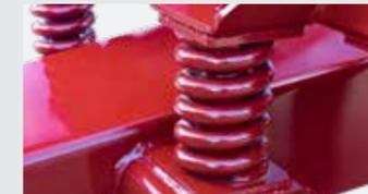
The sprung drawbar reduces shock loading to the tractor towbar, ensuring a smooth power transfer from tractor to trailer and greater operator comfort.
