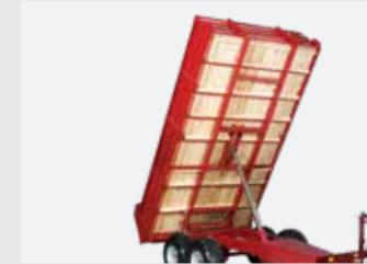
The sides and front are fabricated from 3mm steel plate for strength and rigidity. Sides are hinged so they can be quickly dropped or removed. Giltrap’s simple locking system makes this easy.
