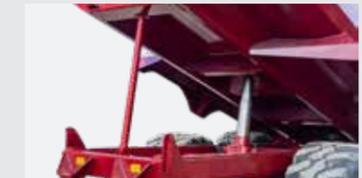
Safety/maintenance stands are fitted as a standard feature. A must when greasing those important pivots or using if the trailer is stored for a length of time to prevent water from ponding in the body.
