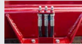
Central greasing is an option on all Giltrap trailers, bringing the centre grease points to an easy access location.
