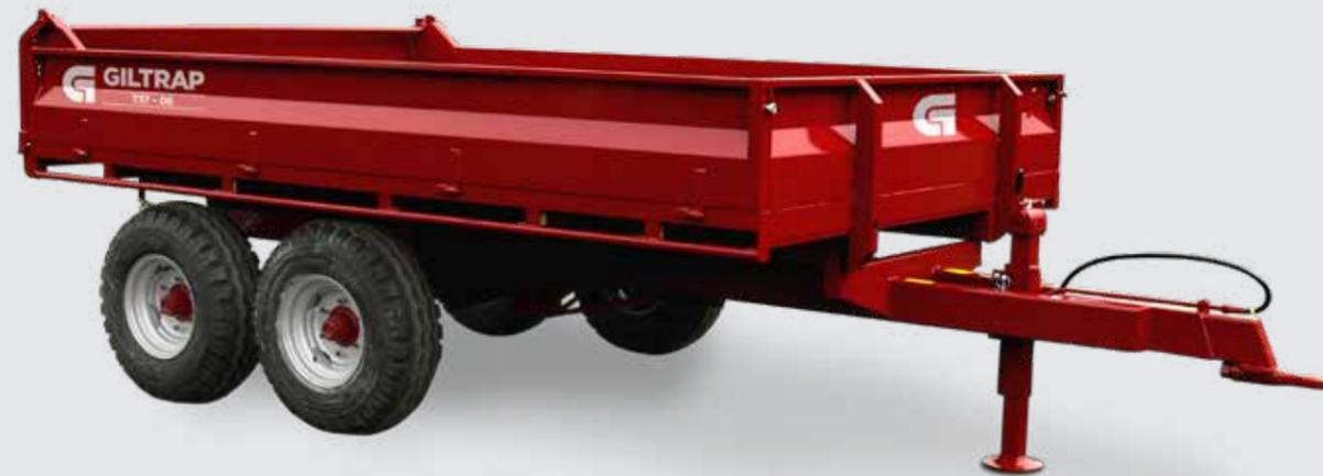
All Giltrap trailers are designed to tip to at least 55° to fully unload, even with wet or sticky products. A single ram, centrally mounted, prevents deck twist.
