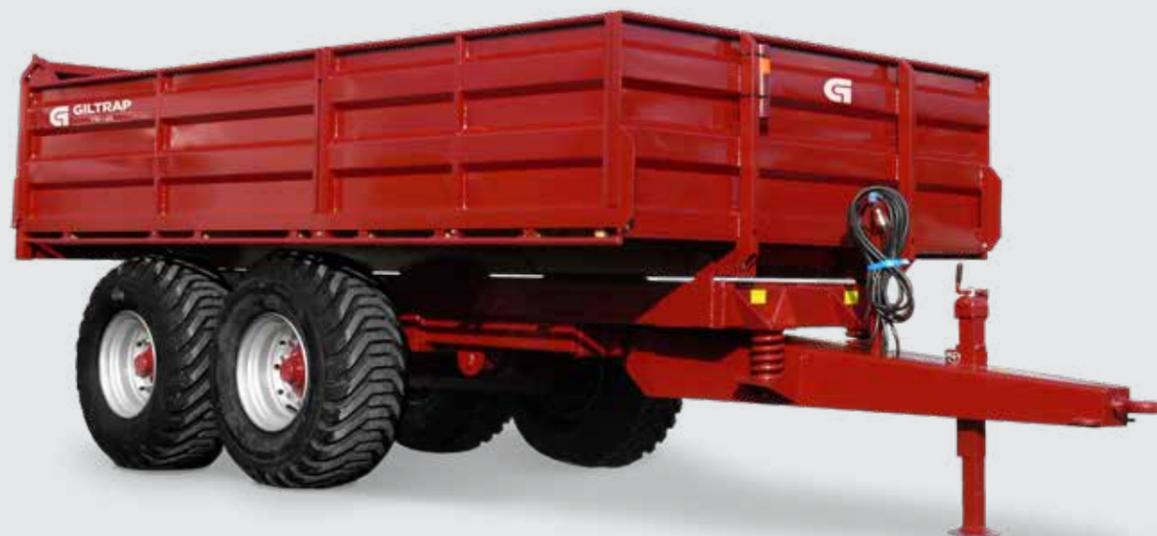
Optional side opening tail door allows for longer loads to be carried without the need to remove the tail door.
