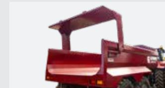
The hydraulically operated, high clearance rear tail door is a standard feature on all construction trailers. The operating rams are well protected and the door can be easily removed if not required.
